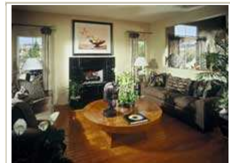
When done right, universal design features in a home are not immediately apparent, says Texas builder Bill Slease. The fireplace in this living room is located off the floor and has no projecting hearth to obstruct access to it when necessary.
